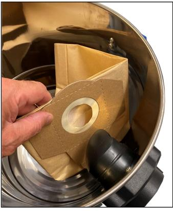
NOTE: In order to ensure proper filtering when vacuuming dust and dry material the intake filter needs removing and the dustbag needs to be put in its place. The intake filter is only to be use vacuuming liquids.
